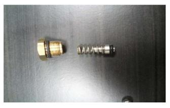
5. <u>Re-insert spring with the shutter back to the valve housing, positioned as shown above.</u>
