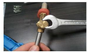
3. Pull the spring and the ball bearing. Check for wear and tear of O-rings and replace as necessary.
